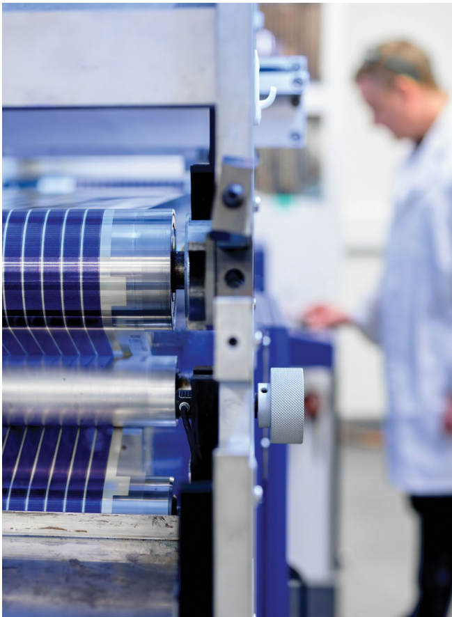
Kardinia Energy’s Printed Solar technology uses carbon-based semi-conducting polymers printed on recyclable PET plastics.
