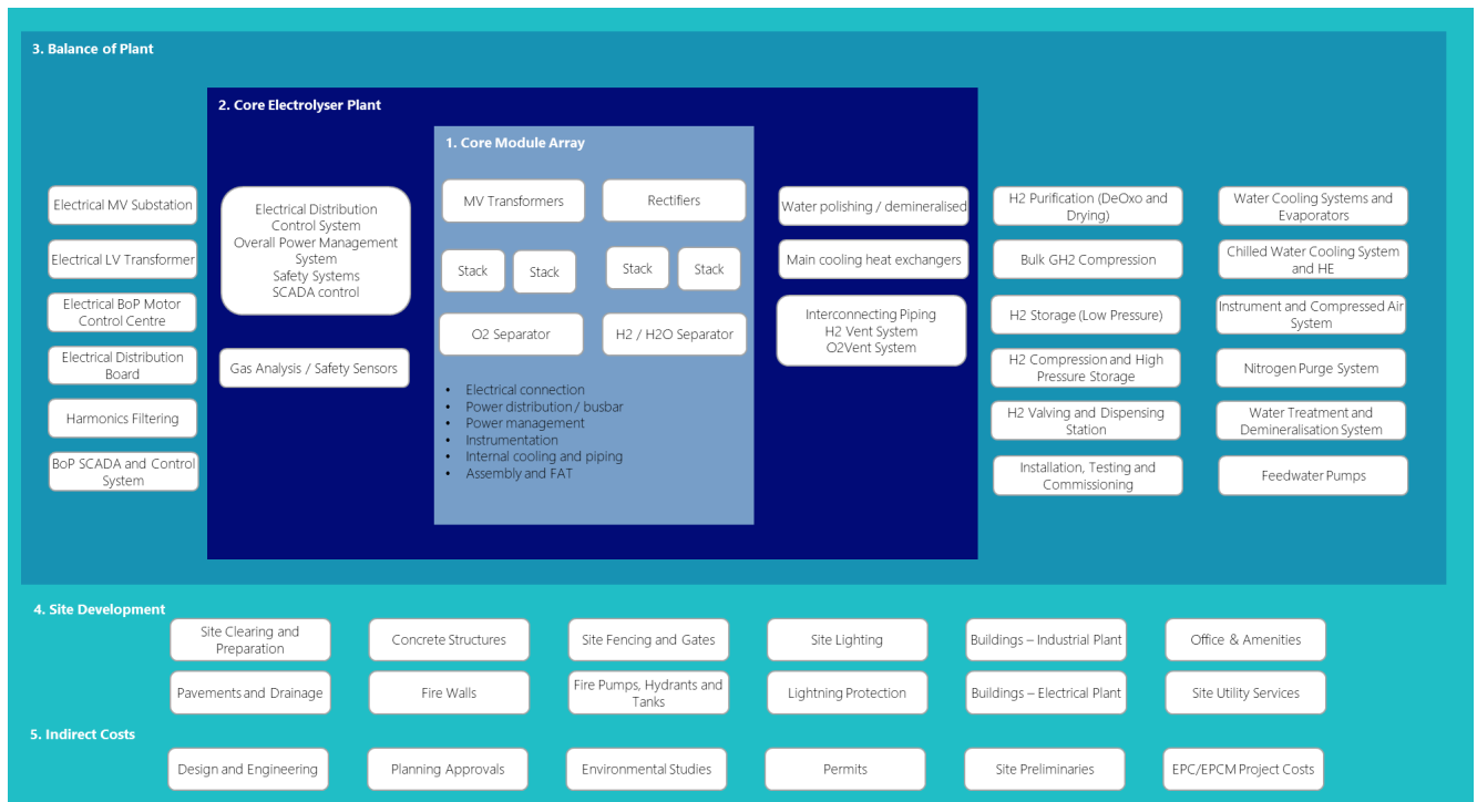
Figure 7: Electrolyser plant components; SOURCE: Arup (2023a), page 30.
