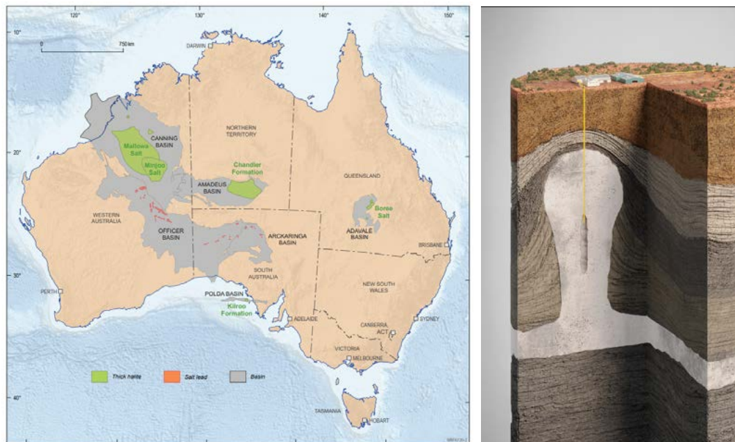
Figure 14: (a) Known thick (>100 metres) underground accumulations of salt (halite) in Australia potentially suitable for large scale hydrogen storage. (b) Example of how underground salt caverns can be used to store hydrogen gas (Geoscience Australia, 2022).
