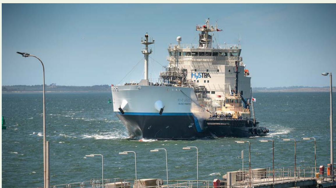
Figure 10: Purpose built vessel known as the 'Suiso Frontier' carrying hydrogen between Australia and Japan.
