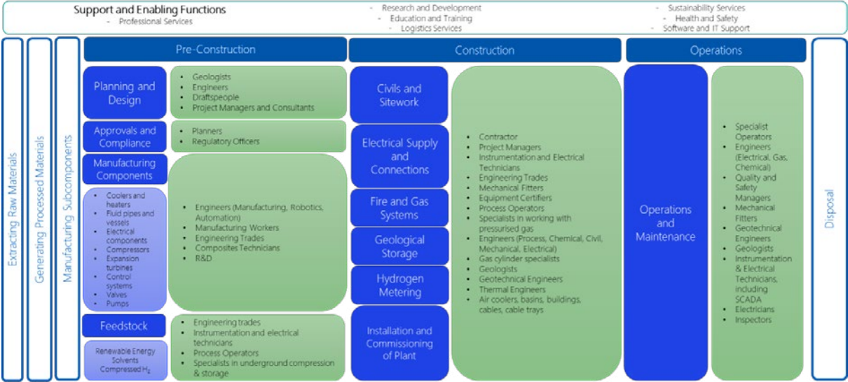
Figure 11 Salt cavern supply chain elements
