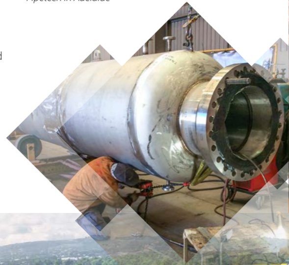
Fabrication of Hydrogen Buffer Storage Vessel for the Hydrogen Park South Australia Project at Pipetech in Adelaide
