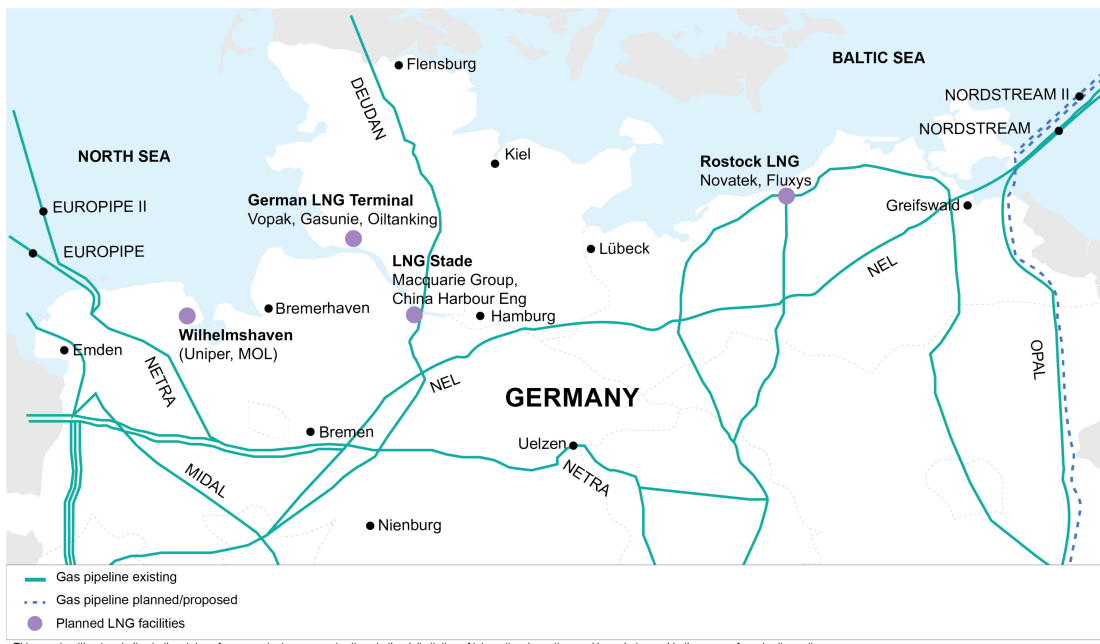
Figure 8.6 Germany's planned LNG facilities
