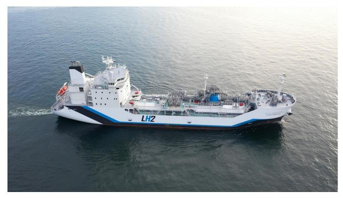
The Suiso Frontier: the world's first liquefied hydrogen carrier. Image: HySTRA
