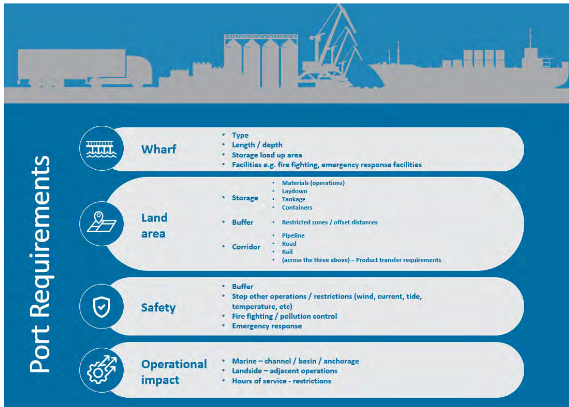
Figure 8 Requirements for hydrogen export ports
